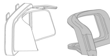
Clean the rubber of the polarisation visor after each use. To disinfect the rubber part remove it from the visor and use medical disinfectant.
